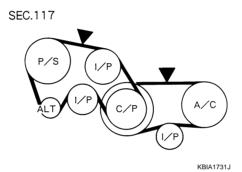
\*: If belt tension gauge cannot be installed at check points shown, check drive belt tension at different location on the belt.
